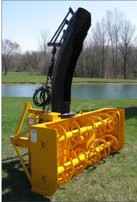
Heavier fan housing Heavier auger tube
