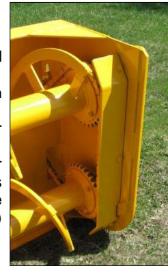
Chain guard Heavier Chain Heavier Auger Heavier Bearings (ductile Housings)
