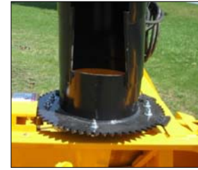
Orbital motor Chute rotator
